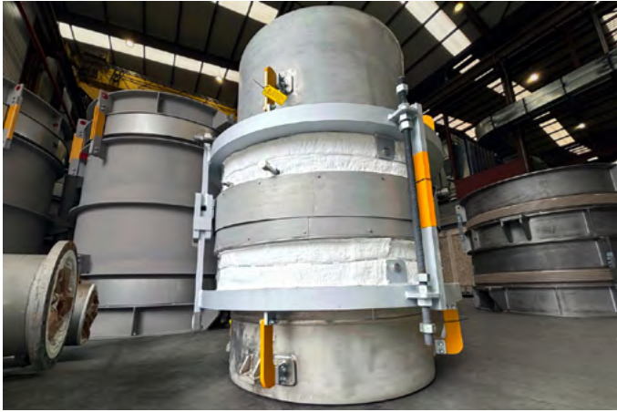
FCC Refractory Lined Expansion Joint for a major Refinery in Scandinavia
