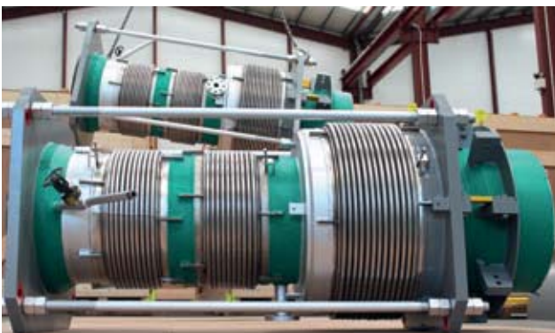
Flexicracking Unit Reactor In Line Pressure Balanced Expansion Joint Two ply monitored bellows Design temperature: 566 °C (media)
