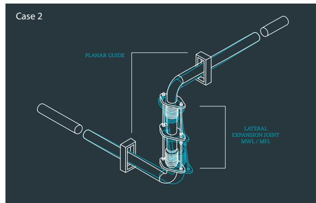
This case shows how an MWL or an MFL Expansion Joint can be used to absorb the thermal Expansion in a Z-shaped section of piping which occurs in three different directions. The fact that this type of Expansion Joint is capable of absorbing lateral movements in more than one direction means that two horizontal pipes can form any angle in that plane.
