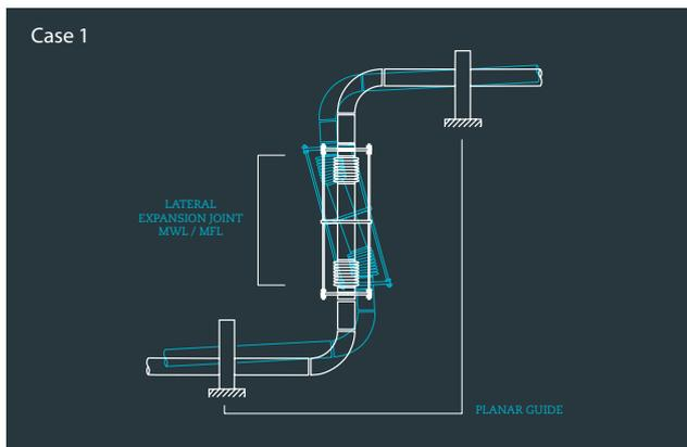
This case illustrates how one MWL or MFL Expansion Joint can be used to absorb the thermal Expansion in a Z-shaped section of piping which only occurs in one plane.
