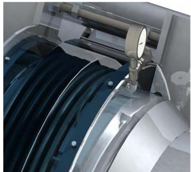
Monitoring system detail with pressure gauge
